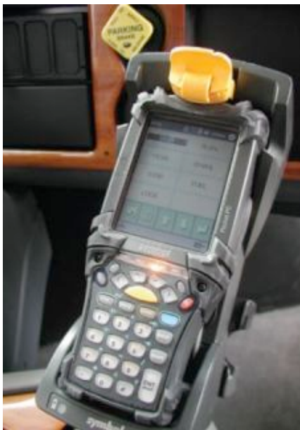
This handheld device from XATA allows companies to monitor fuel and access their drivers’ log digitally.
